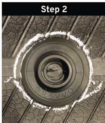
Step 2 Outline dock with tire chalk to define area that will be prepped for proper Dock installation. Cover at least the circular area will the Dock will be installed. Area does not have to be a circle but must enclose the Dock's installation area.
